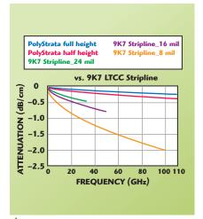
Fig. 12 PolyStrata coax vs. stripline in LTCC.
