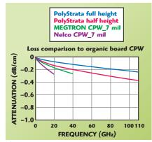
Fig. 9 Attenuation of PolyStrata coax vs. CPW-G on advanced organic materials.
