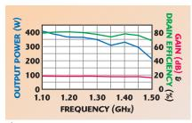
▲ Fig. 1 CGHV14250 typical RF results  $(V_{dd} = 50 \text{ V}, I_{dq} = 500 \text{ mA}, P_{in} = 37 \text{ dBm}, T_{case} = 25^{\circ}\text{C}, Pulse Width = 500 us, Duty Cycle = 10%).$
