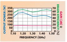
▲ Fig. 3 CGHV14250F CW RF results ( $V_{dd}$  = 50 V,  $I_{dq}$  = 500 mA,  $P_{in}$  = 37 dBm,  $T_{case}$  = 65°C.)
