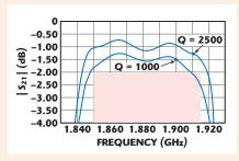
BAW filters offer lower loss and higher Q than SAW filters. These characteristics mean that for challenging applications, BAW filters are often a better choice — even for some frequency bands that are within the range of either filter technology. The diagram here compares the effectiveness of a higher-Q BAW filter (Q=2500) and a lower-Q SAW filter (Q=1000) for the same frequency band (Band 25 TX).
