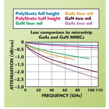
Fig. 10 Attenuation of PolyStrata coax vs. microstrip on GaAs and GaN.
