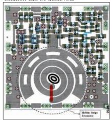
▲ Fig. 14 Layout of 10 GHz oscillator (depicts the phase-injection-mode-locked) Möbius strips resonator (22 mil substrate thickness with 2.22 dielectric constant, 0.7" × 0.75" × 0.18").
