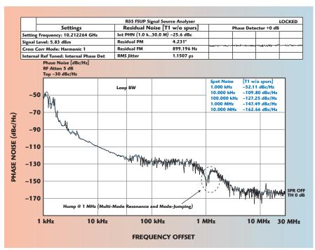
Fig. 12 Measured phase noise plot of 10.2 GHz MCEMR VCO.
