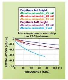
Fig. 8 Attenuation of PolyStrata vs. microstrip on Alumina.
