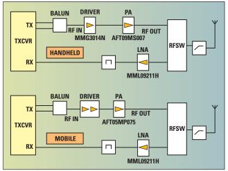
Fig. 2 Typical circuits for handheld and vehicle-mounted radios using these new devices.
