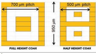
Fig. 2 Cross-sections of full and half height PolyStrata coax.
