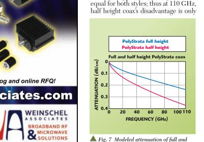
Fig. 7 Modeled attenuation of full and half height PolyStrata coax.
