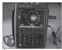
Fig. 18 Agilent FieldFox RF analyzer N9912 with the device connected — the Smith Chart indicates the broadband coupling of signal into the device. <sup>14</sup>
