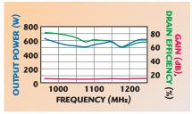
Alpha Fig. 4 CGHV14500F in applications circuit (V<sub>dd</sub> = 50 V, I<sub>dq</sub> = 500 mA, P<sub>in</sub> = 41 dBm, T<sub>case</sub> = 25°C, pulse width = 500 μs, duty cycle = 10%).
