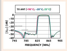
Temperature drift has become an important issue as spectrum becomes more crowded and high selectivity is required to minimize insertion loss and ensure rejection of adjacent bands.
