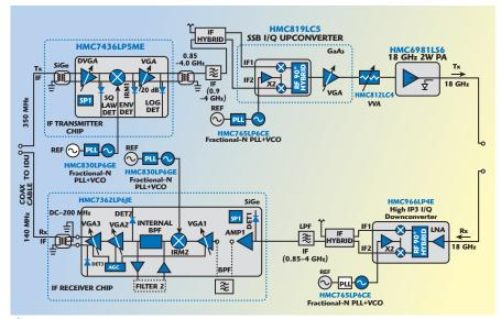
Fig. 1 Complete 18 GHz transmit/receive chipset reference design.
