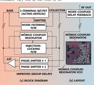
▲ Fig. 13 Shows the typical block diagram 10 GHz Möbius coupled resonator VCOs using a SiGe HBT active device, built on 20 mil substrate material.
