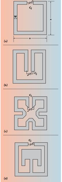
▲ Fig. 7 Typical layout of a tunable square open loop resonator: conventional square open loop hairpin resonator (a), folded arms square open loop resonator (b), meander line square open loop resonator (c), dual mode square open loop resonator (d). 36
