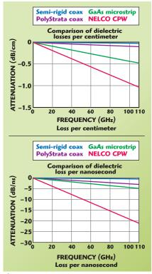
Fig. 4 Loss tangent attenuation for various transmission lines.
