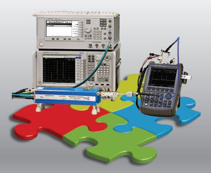
With a single connection, measure S-parameters, Gain Compression and Intermodulation Distortion (IMD).
