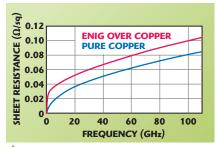
▲ Fig. 5 Comparison of surface resistivity for ENIG over copper (1 µm gold over 1 µm nickel) and pure copper.
