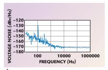
Fig. 5 Voltage noise at the phase detector output.
