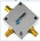
The 3 port 180 degree hybrid, model DJK-2120, covers a wide frequency range of 20 to 1200 MHz (BW 60:1) with excellent performance. It is built in a rugged
