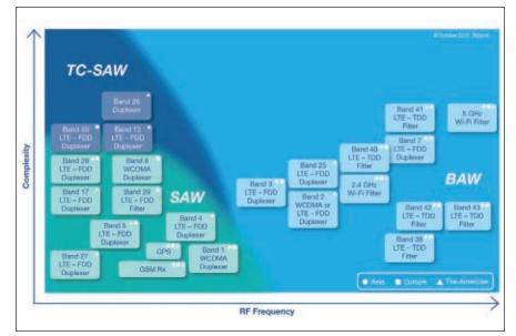
Fig. 2 Matching filter technologies to applications.
