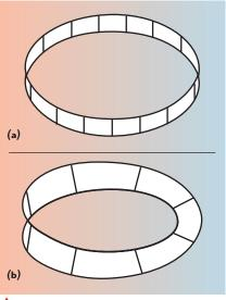
▲ Fig. 4 Typical closed loop ring resonator (a) and the Möbius strip resonator (b) a topological transformation of ring resonator into a Möbius strip resonator.<sup>15</sup>
