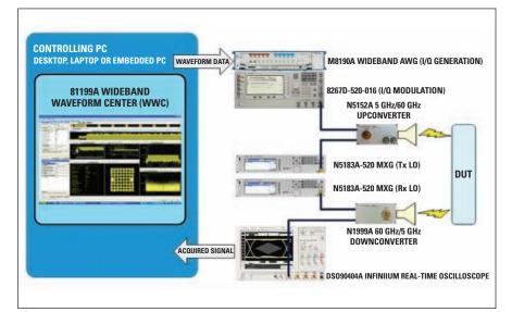
lacktriangle Fig. 5  $\,$  802.11ad physical layer signal generation and analysis solution.
