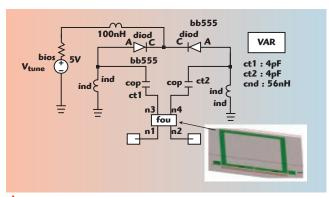
▲ Fig. 8 A typical setup for carrying out the measurement of the transmission coefficient  $S_{21}$  ( $\omega$ ) for analyzing the coupling characteristics of the varactor loaded tunable open loop resonator.
