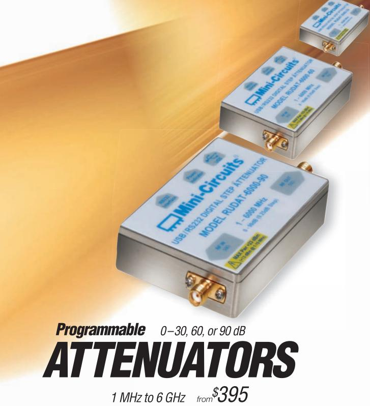
Mini-Circuits RUDAT-6000 series **USB** controlled digital step attenuators support frequencies from 1 MHz to 6 GHz in versions with maximum attenuation of **30**, **60**, and **90** dB with **0.25** dB attenuation steps, providing precise level control for a wide range of test applications. All models achieve accurate, repeatable performance in a miniature, shielded metal case (2.0 x 3.0 x 0.6"). Our
