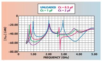
$\blacktriangle$  Fig. 9 A CAD simulated (Ansoft Designer) plot of  $S_{21}\left(\omega\right)$  of a varactor loaded open loop resonator for different capacitance values.
