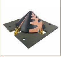
Fig. 5 LDS antennas offer full 3D shaping for maximum design freedom (Image: Leibnitz University Hannover, C.Orlob).
