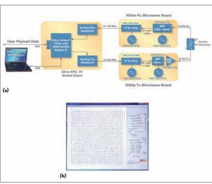
Fig. 4 18 GHz microwave link demonstration setup (a) and constellation view (1024-QAM).
