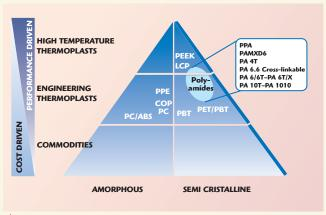
Fig. 1 The material range of deliverable LDS plastics.
