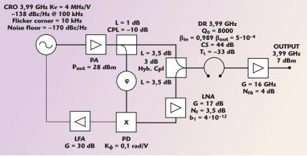
Fig. 4 Oscillator stabilized by a frequency discriminator.
