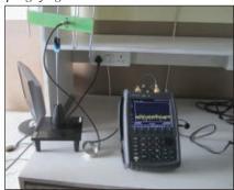
▲ Fig. 19 The VNA was switched to cable and antenna testing mode to check the delay response in real time of the Möbius strips shown in Figure 16. <sup>14</sup>
