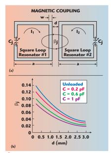
Fig. 6 A typical capacitive loaded magnetic coupled square loop resonator layout (a) and plot of magnetic coupling  $\beta_i$  (b).
