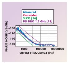
▲ Fig. 8 Measured and calculated phase noise compared with a DRO and SLCO.
