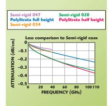
Fig. 11 Attenuation of PolyStrata coax vs. semi-rigid coax.
