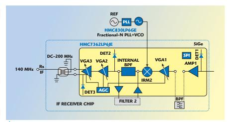
📤 Fig. 3 HMC7362LP6JE IF receiver chip block diagram.
