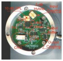
Fig. 7 Oscillator assembly.
